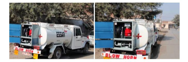
EAST-MAN 12V DC Mobile Fuel Dispensing System is a self contained, demountable fuel dispensing unit which has been designed to meet the needs of fuel distributors who's customers require low volume 'Metered' deliveries of fuel into plant equipment, building sites, generators, boats, green houses and other sites which may have difficult access and where it may not be cost effective or practical to send a conventional fuel delivery tanker.
