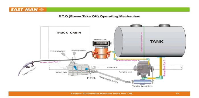
EAST-MAN products to make a functional Diesel Bowser. PTO Driven Diesel Bowser is a self contained fuel dispensing unit which has been designed to meet the needs of fuel distributors who's customers require 'Metered' deliveries of fuel into plant equipment, building sites, generators, boats, green houses etc.
